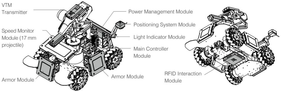
Connection reference for each module on the Robot Side
